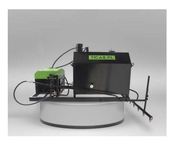
The bitumen emulsion sprayer BS- 500, 1000 is intended for priming before asphalt laying, asphalting of adjacent territories, as well as for filling seams and cracks with bitumen emulsion. The bitumen emulsion is supplied from a tank with a volume of 500 or 1000 liters. The heating system allows you to use a spray of bitumen emulsion in the cold season. Easy to use. It has its own system rinsing. It is made on a frame, or mounted on the trailer.
